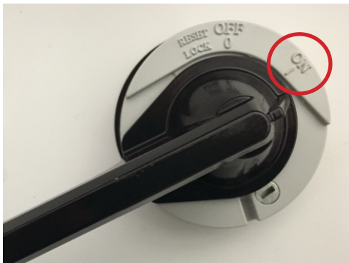
2. MAIN POWER SWITCH in ON Position
