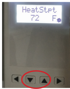
6. Heat MODE Selected - Adjust Temp Set Point
