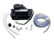
The condensate pump provides for the automatic removal of condensate water during the cooling process. The pump is capable of pumping to a 20 foot height, allowing for the routing of the drain line above the drop-ceiling to a nearby drain. The pump is controlled by an internal float-switch/check valve, which turns the pump on and off automatically. The pump is also equipped with a condensate over-flow safety switch that will shut down the unit compressor when the pump is not working properly.
